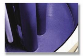
Because A. O. Smith applies PermaGlas® Ultra Coat™ after the tank is welded, there is no chance of "weld burn" that can burn away normal glass lining and expose bare steel to water.
