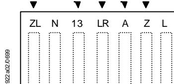
Terminals to RAST5 standard, also suited for use with quick connectors to DIN 46244-A 6.3-0.8
