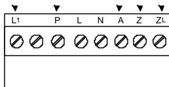
Screw terminals for single-wire cables up to 2.5 mm<sup>2</sup> (AWG12)
