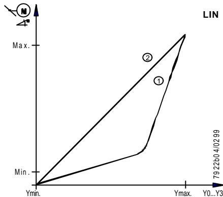
By setting shorting plug «J1» to position «1», the proportional behavior of the actuator (curve ②) can be matched to the control (curve ①). In the case of small signals, linearization of the angle of rotation produces overproportionally small angular changes and, in the case of greater signals, overproportionally large angular changes. Used in connection with non-linear regulating units, such as air dampers.
