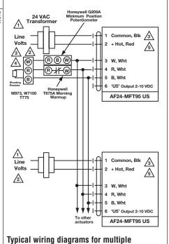
actuators used with the W973, W7100 and
