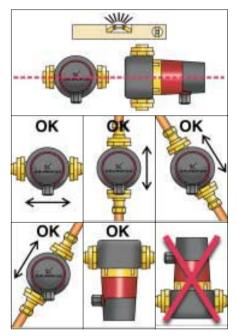
It is preferred that the circulator always remains in a horizontal position. It is acceptable for the circulator to be mounted under the piping in a vertical position. The circulator cannot be mounted over the piping in a vertical position.
