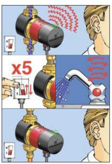
The timer is a 24-hour AM/PM timer with 20-minute interval. For ease of programming the timer head can be swiveled stop to stop almost 360 degrees.
