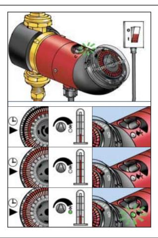
In the unlikely event that instant hot water is not available, the circulator impeller may be blocked by calcium/sediment deposits. Follow these steps to clean the impeller:
