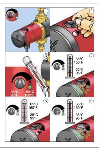
When the timer and thermostatic controls are used together, the circulator operates **ONLY** at the programmed timer settings **AND ONLY** when the temperature conditions of the aquastat have not been met.
