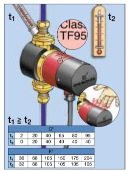
The liquid temperature must always be greater than the ambient temperature to avoid condensation. The table shows the maximum allowed ambient temperature for a given liquid temperature. The maximum allowable fluid temperature is 204 deg F.
