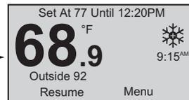
**Temporary Hold** – Select the time when the hold will end. Select **Accept**. The **Main Menu** will appear. Select **Back**. The main screen will show the hold temperature and time. When the hold expires, normal operation continues.
