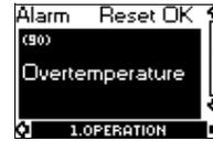
If the pump is faulty, the cause will appear in this display.
