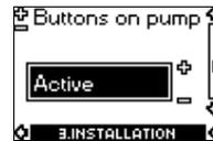
To prevent unauthorized persons from operating the pump, the function of the buttons (⊕), (⊖) and (⊙) can be deactivated in this display. The buttons can be reactivated only with the R100.
