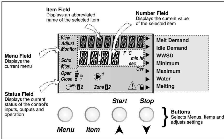
The tekmar Snow Detector & Melting Control 664 has a Liquid Crystal Display (LCD) and four push buttons (**Menu**, **Item**, **▲**, **▼**) which are used to view and adjust the settings.
