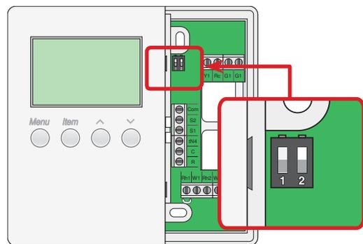
**Note:** The tN4 System Control's Lock/Unlock DIP switch overrides the Lock/Unlock DIP switch on the 545. Set the tN4 System Control's Lock/Unlock DIP switch to the Unlock position before Access Levels can be changed on the thermostat.
