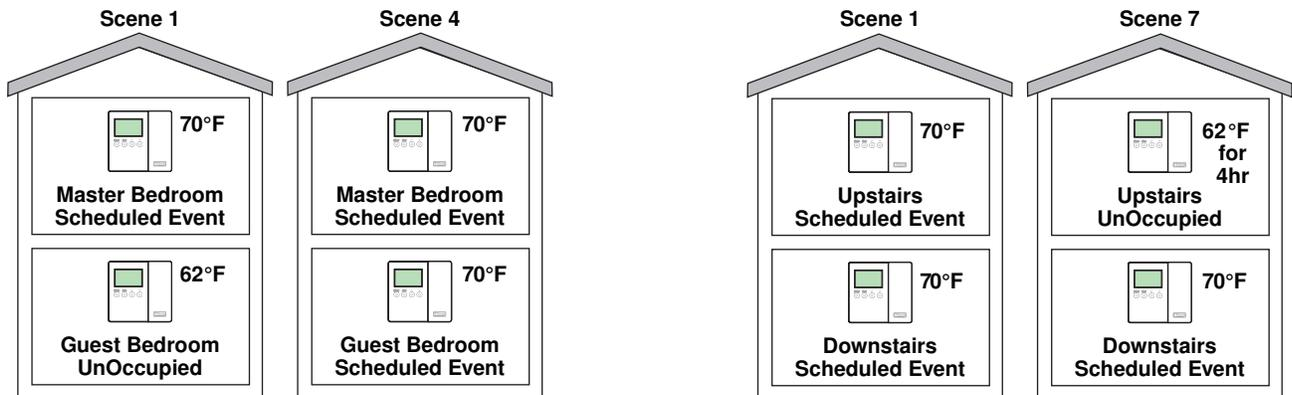
To set the temperature while the occupants are away, use the Permanent Away 2 scene. This scene changes all thermostats on the network to the Away temperature setting. If there is an Outdoor Reset Module on the tN4 communication bus, the boiler no longer responds to domestic hot water calls for heat. Setpoint demands continue to operate as in the Occupied mode.
