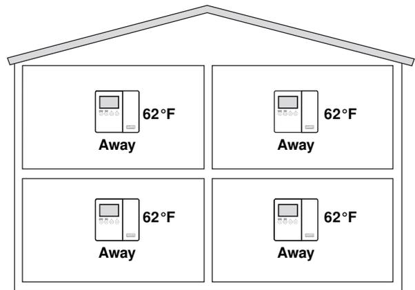
Use the Radiant Base Load feature when operating radiant floor heating in conjunction with a fast acting secondary heat source. The Radiant base Load feature is only available when a floor sensor is not installed. A time lag occurs with radiant floor heating due to the large thermal mass of concrete floors. This effect is evident when the thermostat temperature setting is increased and the radiant floor takes a while to reach the specified temperature.
