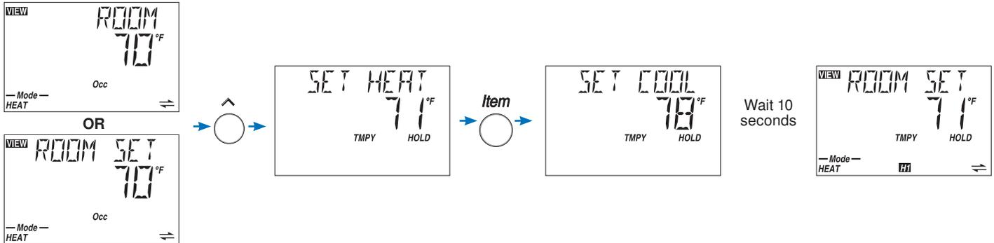
By default, the temporary change lasts for 3 hours. This duration can be changed by going to the “Temporary Zone Hold” item in the Scene menu.
