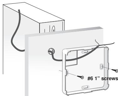
**NOTE:** If the 508 is to be used for remote sensing (i.e. The built-in air sensor is disabled and an indoor sensor is being used.) Mount the thermostat in the desired location in an appropriate manner.
