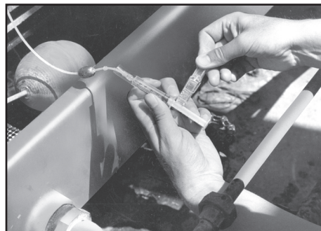
Use syringe to charge Drip Feeder.
