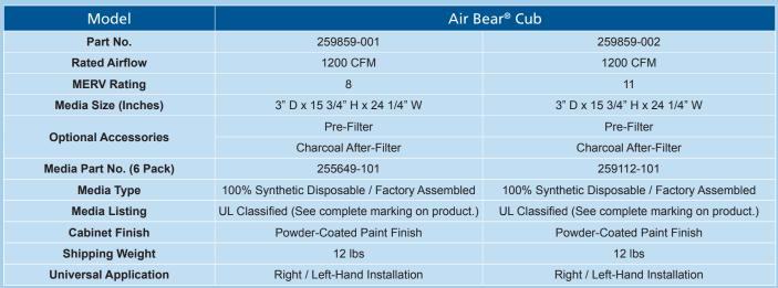
Air Bear® Air Cleaners have been tested using ANSI / ASHRAE 52.2-2007 standard test procedures.
