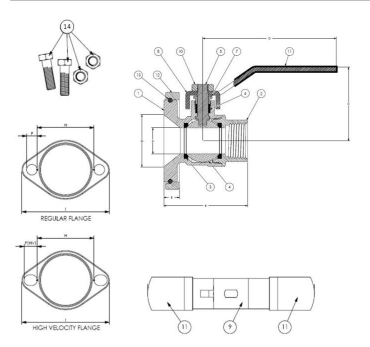
**Specifications**: Designed for residential, commercial or industrial use with water or a glycol mixture. This approved Webstone valve is actuated by a blowout proof stem and features an adjustable packing gland. Flange features a conical inlet to minimize turbulence. The rotating flange is secured by a snug-fit snap-ring that provides greater control over positioning during installation. Threaded ends comply with ANSI B1.20.1.
