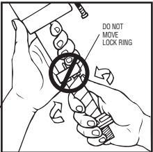
Adjust height of fill valve by turning lower shank in or out of the valve body. Do not move lock ring. It holds the valve body and shank together under pressure. Do not interchange body with old shank, as leaking can occur.
