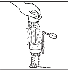
Flushing Out the Debris: Hold a cup over the uncapped valve to prevent splashing. Turn water supply full on and off a few times. Leave water supply off. Check for leaks. Tighten nuts just enough to stop leaking.
