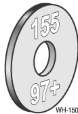
Figure 11 Propane gas orifice identification WM97+155
