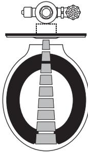
2. As the user enters the beam's effective range (22" to 42") the beam is reflected into the OPTIMA Scanner Window and transformed into a low voltage electrical circuit. Once activated, the Output Circuit continues in a "hold" mode for as long as the user remains within the effective range of the Sensor.
