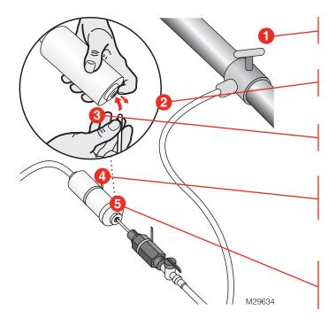
Turn the water supply off at the saddle valve or T-fitting and manual shutoff valve.
