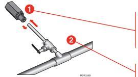
Connect one end of the remaining length of water line to the backflow preventer. Apply a modest pull to ensure a tight fit. See "Reverse Osmosis Filter" on page 23 if using the Reverse Osmosis Filter.
