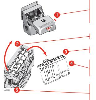
Remove TrueSTEAM cover and inspect water level sensor. If debris buildup is present, clean with recommended cleaning agent. If cracks or visible discoloration is noticed, replace sensor (see below).
