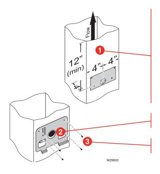
Position the template on the supply duct:
