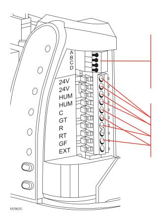
Use the terminals (found inside the cover) to wire TrueSTEAM to the humidity control and the HVAC system.
