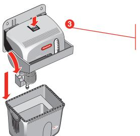
Grip the tank bottom firmly. Push down the safety release button and pull the latch forward to release the tank.
