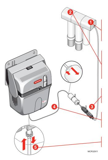
Do not use hot water supply. Cold water is required to cool boiling water to safe draining temperatures.
