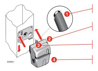
Make sure the foam gasket is positioned correctly over the nozzle.
