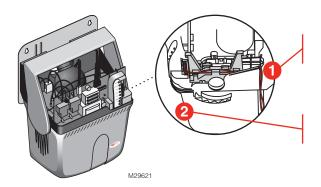
Route wires through the raised tabs and out the notch at the rear of the chassis.
