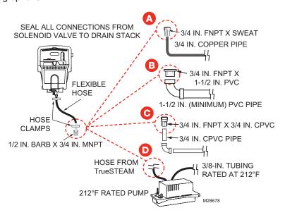
Option 1: Plumbing to drain with condensate pump.
