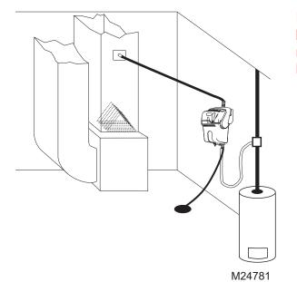
Note: If air handler location temperatures will drop below freezing at any time, TrueSTEAM must be mounted in a conditioned space, running a remote hose to the duct.
