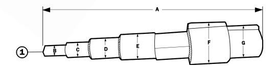
**Specifications:** Designed for use with a radiator valve union tailpiece connection. This heavy duty tool is used internally to securely tighten any union tailpiece to a radiator and fits valve sizes ½" to 2".
