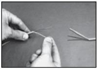
**Step 2.6.** Pull the braid shield to make into a pigtail.
