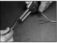
**Step 2.7.** Use thermal wire strippers to remove ½" of the insulation from the heating wires.
