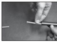
**Step 2.2.** Slide the outer shrink tube over the longer cable lead.
