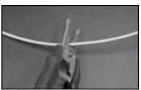
**Step 2.1.** Cut out a 2" to 3" section of the heating cable to remove the damage.
