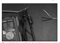
**Step 2.8.** Use a digital multimeter and a TDR to test from this location. Check for any additional cable damage by "looking" down the cable in both directions. For assistance in using these test instruments, consult the instructions that came with them or contact Watts Radiant.
