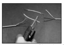
**Step 2.10.** Remove  $\frac{1}{2}$ " of the insulation from both ends of the jumper wires.
