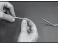
**Step 2.4.** Push the braided shield back to loosen it.
