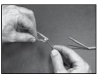
**Step 2.5.** Use a small screwdriver, or similar, to make an opening in the braid shield. Pull each wire through the braid shield.
