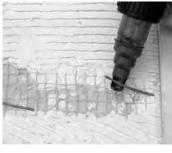
**Step 4.4.** With either type of jacket, if the jacket slug doesn't easily pull off you may need to use your heat gun to gently warm the slug, which should soften and loosen it for you. Use the heat gun (set to about 500°F) and move the gun back and forth under the jacket slug for about 3 or 4 seconds, or until it can be easily removed.
