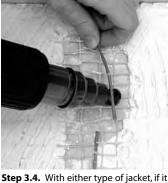
Step 3.4. with either type of jacket, if it doesn't easily pull off you may need to use your heat gun to gently warm the slug, which should soften and loosen it for you. Use the heat gun (set to about 500°F) and move the gun back and forth under the jacket slug for about 3 or 4 seconds, or until it can be easily removed.
