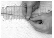
**Step 4.6.** Loosen the braid by pushing back on the braid about 1/2," causing the ends of the heating wires to be exposed.
