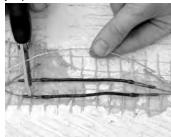
**Step 4.19.** If necessary, cut the ground jumper wire shorter so that it overlaps the ends of the ground braid lead wires by about 1/2" to 3/4".
