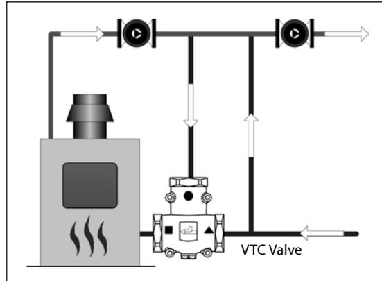
Because gravity conversion systems contain an enormous volume of water, the water returning to the heat source could be significantly cooler, leading to condensation and a shorter life for the heat source. Adding a thermic valve to the system will prevent the boiler from sustained operation at temperatures below the dew point of their flue gases.
