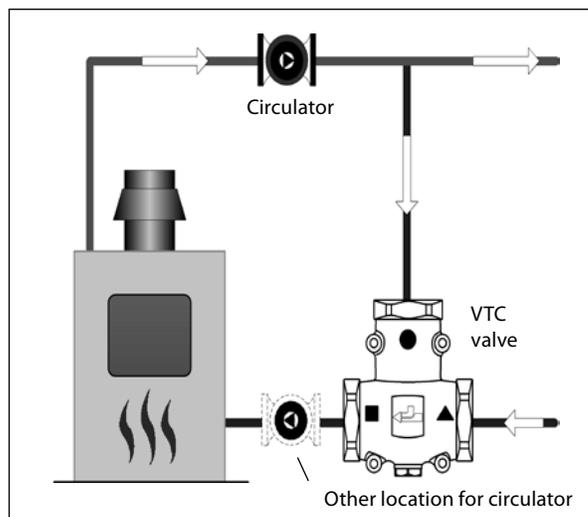
The VTC valve, when placed on the return side will open when the minimum return temperature of the element is reached. When the fluid temperature reaches 18°F (10°C) higher than the element's temperature, the return port from the system will be fully open.
