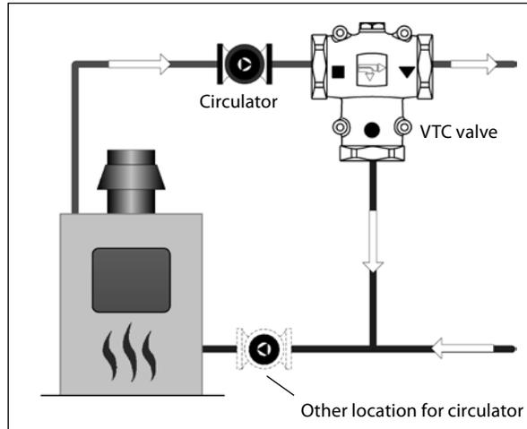
When the VTC is piped on the supply side out from the heat source, the valve will begin to allow water out to the system when the temperature of the fluid meets the temperature of the inserted thermostat element.
