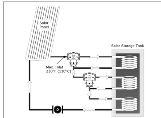
With the thermic VTC valve, an efficient method of charging a tank can be done. To achieve efficiency through the solar panel, cool water should enter allowing for a higher differential temperature across the panel. Additionally heated fluid from the panel should be properly distributed within the tank to reduce stratification i.e. even temperature distribution, within the tank.
