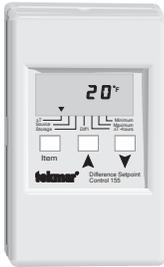
The Difference Setpoint Control 155 is a microprocessor-based control that allows the transfer of heat from a source to a storage tank whenever the temperature difference between the two is greater than the selected  $\Delta T$  setpoint. Additional setpoints are also included to help prevent the storage tank from overheating or the source from freezing. Both drainback and draindown systems can be used with this control.
