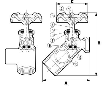
**Specifications:** Designed for residential, commercial or industrial use in hydronic heating systems. Threaded ends comply with ANSI B1.20.1.
