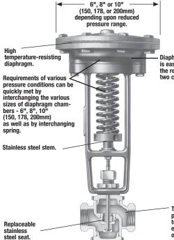
Diaphragm chamber is easily changed by the removal of two cap screws.
