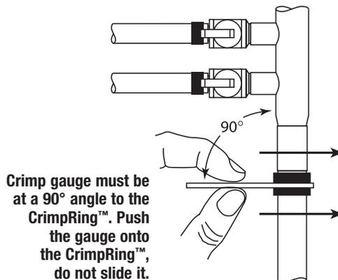
**Crimp gauge must be at a 90° angle to the CrimpRing™. Push the gauge onto the CrimpRing™, do not slide it.**
