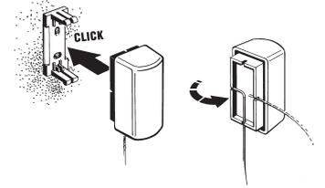
Attach the sensor bracket to the desired location. Pull out the required length of capillary tube and secure to the sensor as shown. Push the sensor onto the base.
