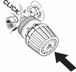
Push the thermostat firmly onto the valve until an audible "click" is heard.
