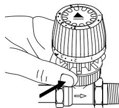
Once the thermostat is mounted on the valve, push in the theft protection device. The thermostat cannot be removed.
