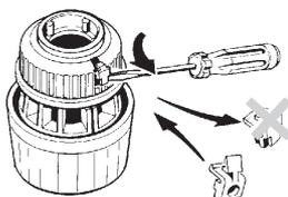
Remove the cover and install the theft protection button, code 013G5245 (20 pcs) without pushing it all the way in.
