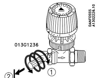
To remove the theft protection use screwdriver 013G1236 and screw into the hole (1). Pull out until the stop is reached (2).
