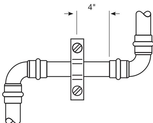
Figure 3.2 Spacing for sliding pipe hanger
