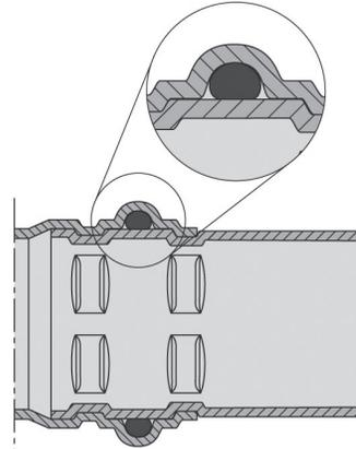
Viega fittings are pressed before, after and on top of the sealing element in a single step, which creates a permanent connection that is secure and guaranteed to last.
