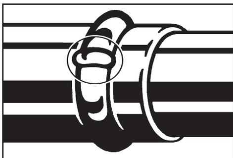
When the fitting is pressed (Figure 1.3), a permanent, sealed, non-detachable, mechanical connection is created.
