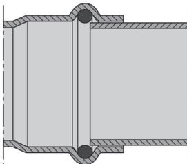
4. All Viega ProPress fittings are designed with cylindrical pipe guides to keep the pipe straight and protect the sealing element during assembly.
