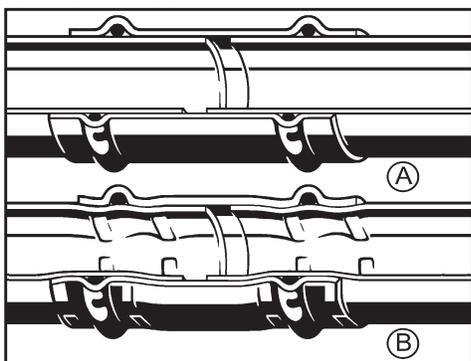
Unpressed fittings from other manufacturers, without the patented Smart Connect feature, may not leak during the initial system pressure test. However, they can unseat in future system operation. The Smart Connect feature is designed to protect from this potential risk.
