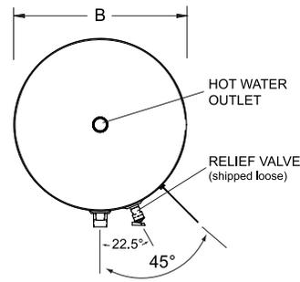
The "Hot Water Outlet" connection is Female NPT.
