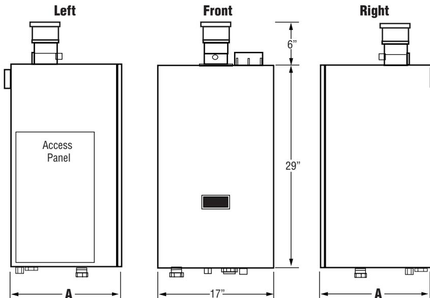
NOTE: Combi kit extends 13" below boiler, with all connections on left side
