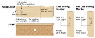
No notching or boring into top/bottom flange portions is allowed. 11/2" hole allowed anywhere along web. Folow all I-Joist manufacturer's instructions.
