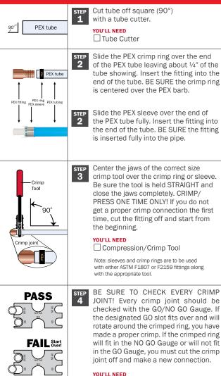
BE SURE TO CHECK EVERY CRIMP JOINT! Every crimp joint should be checked with the GO/NO GO Gauge. If the designated GO slot fits over and will rotate around the crimped ring, you have made a proper crimp. If the crimped ring will fit in the NO GO Gauge or will not fit in the GO Gauge, you must cut the crimp joint off and make a new connection.
