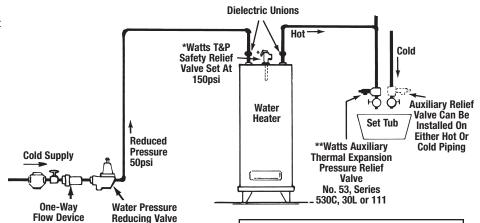
\*T&P valve should be set according to tank working pressure or local code requirements.
