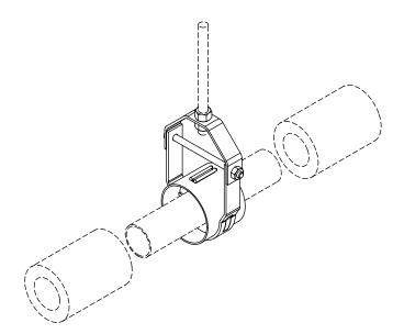
THE HOLDRITE® Insulation Coupling Clevis System Hanger provides ideal support for insulated pipe lines. These clevis hangers allow insulation to but up to each side of the insert and eliminate the need for rigid insulation inserts or insulation shields.
