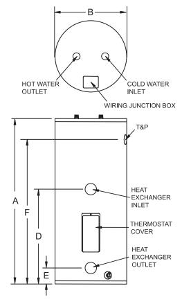
**NOTE:** The uniform plumbing code limits the boiler pressure relief valve to 30 psi when installing in a potable water system.
