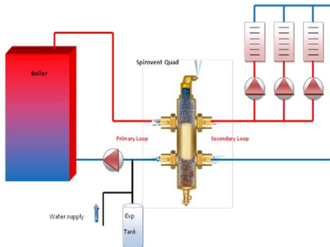
Units must be mounted in straight runs of horizontal piping in a perfectly upright position to allow the vent to operate freely. The piping normally supports the weight of the Spirovent units up to and including 12". Support legs recommended for units 14" and larger. "X" pipe diameters of straight run before and after the unit are not required.
