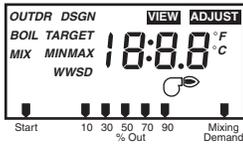
The control then automatically goes to operating mode, and displays the outdoor temperature.
