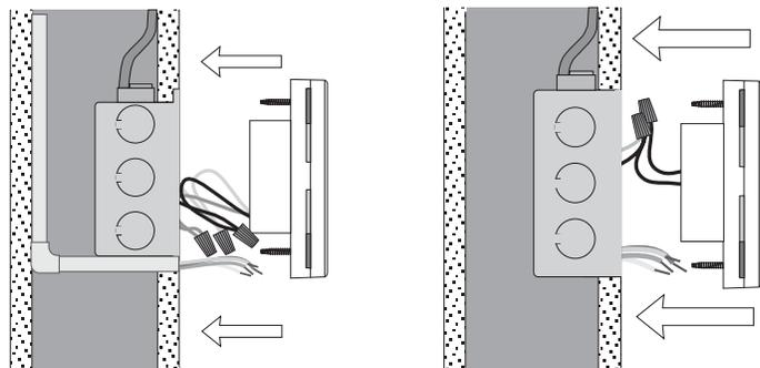
The variable speed injection pump and system pump wiring terminates in the electrical box. All other electrical wiring terminates in the two wiring chambers on the control. The wiring is roughed-in to the electrical box prior to installation of the control.
