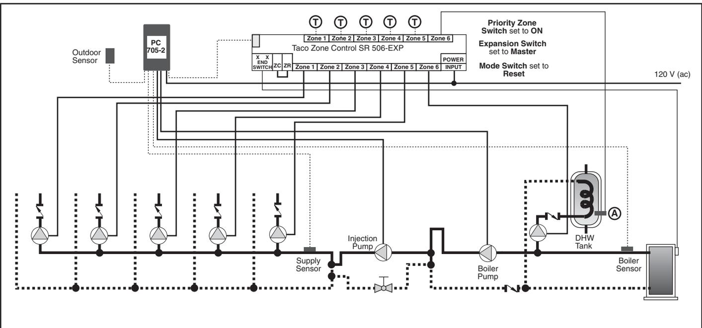
Drawing 3/705-2: Radiant Floor Heating, High Temperature heating with DHW generation
