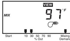
**Mixing Target Temperature**
