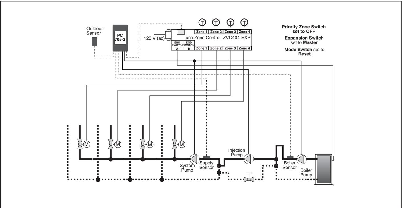
Drawing 2/705-2: Radiant Floor Heating with DHW generation
