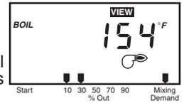
To view all control settings, the Item button may be pressed and held while in the View Menu. The control will then scroll through all the adjustable items.
