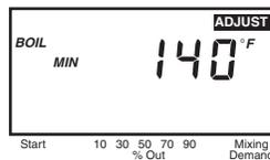
The control automatically goes back to viewing when the buttons are left alone for 20 seconds
