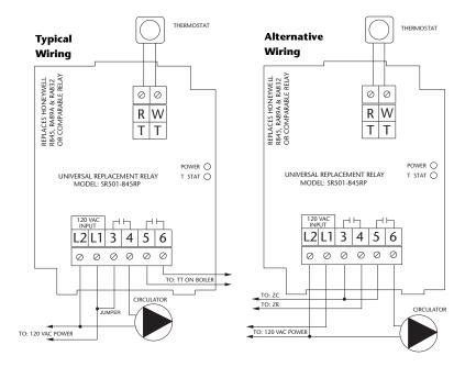
**Note:** When using Alternative Wiring diagram, the boiler operating control's ZC terminal will see the load of the circulator(s).
