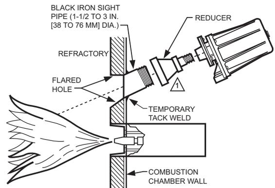
IF VENTILATION OF THE SIGHT PIPE IS REQUIRED, ADD PIPE TEE, PERFORATED NIPPLE, OR OTHER SUITABLE DEVICE FOR VENTILATION.
