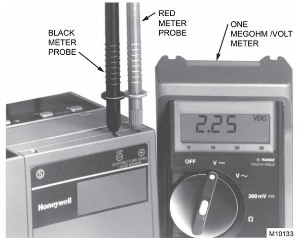
Fig. 11. Measuring voltage flame signal with 7800 Series controls.
