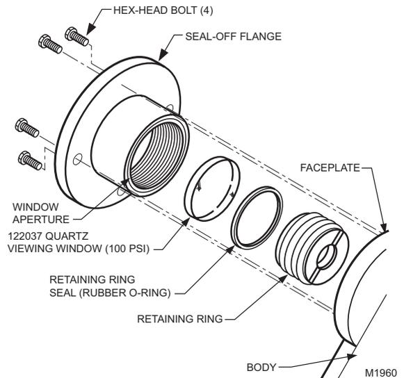
**Fig. 13. Replacing quartz viewing window on C7961F.**
