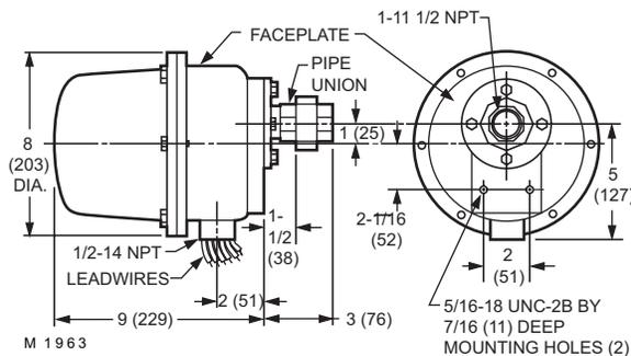
Fig. 2. Dimensions of C7961F in in. (mm).
