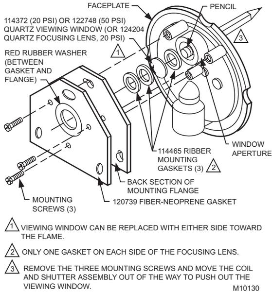
**Fig. 12. Replacing quartz viewing window or focusing lens.**
