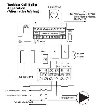
**Operation:** When the thermostat calls for heat, the appropriate circulator is energized and the isolated end switch (X and X) will start the boiler. Priority Output has power all the time, except when the thermostat is calling.
