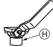
**Be careful not to tip the valve as its components might fall out.** If this occurs, reassemble as shown (J).
