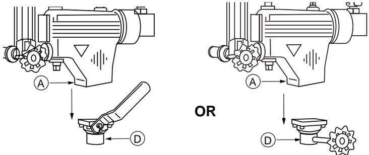
NOTE: For spring type blow down valves, the spring mechanism must be removed from the control body.
