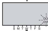
"OCC" will be flashing. Allow control to time-out or press "Menu", and control will be in Occupied override. The normal program will resume at the start of the next Occupied event
