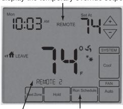
The name of the remote sensor will be displayed. In this example, it is **REMOTE 2**.
