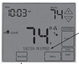
**NEXT ZONE** key cycles through ambient temperatures for connected zones.
