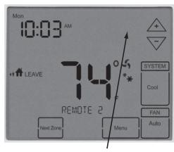
Setpoint will only be displayed for the zone currently being used by the program or in hold. Press the  $\triangle$  or  $\checkmark$  to show the setpoint for adjustment.
