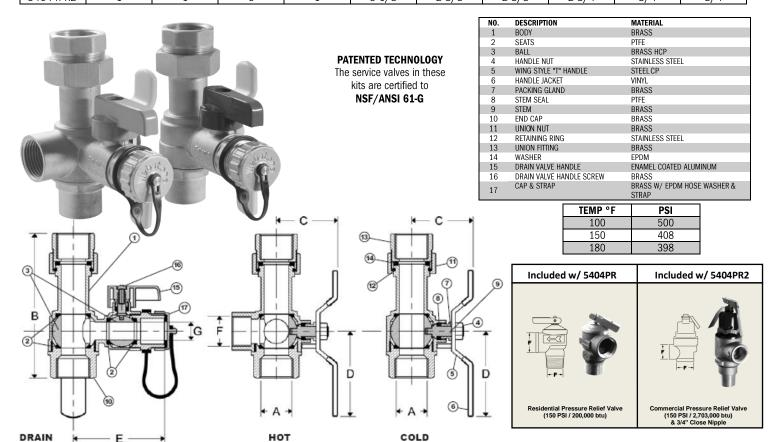
**Specifications:** Designed for residential or commercial use with potable water. This approved Webstone valve is actuated by a blowout proof stem and features an adjustable packing gland. Solder joint temperature ratings are per ASME B16.18 Annex A for 95-5 solder. Other solder materials have lower pressure/temperature limits. Do not silver braze or overheat valves when soldering.
