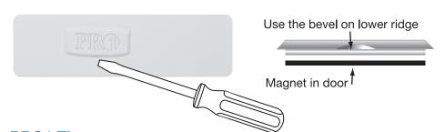
Gently slide a screwdriver into the bottom edge of the badge. Gently turn the screwdriver counter clockwise. The badge is held on by a magnet. The badge should pry off easily. **Do not use force.**
