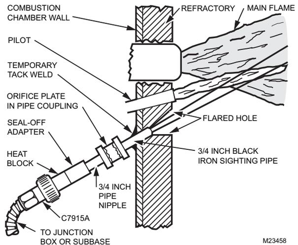
Fig. 9. Mounting C7915A Infrared Flame Detector (and accessories).
