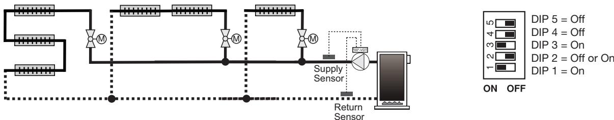
The 00-VDT Variable Speed Circulator adjusts its speed to maintain the differential temperature (based on the RANGE dial setting) between the supply sensor and the return sensor whenever a heat demand is present. This will increase overall comfort and sharply reduce boiler short-cycling. The 00-VDT will also control velocity noise issues in the system, eliminating the need for a pressure differential bypass valve.
