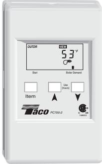
The PC700-2 is a microprocessor-based control designed to regulate the supply water temperature of a single boiler, based on the outdoor temperature. A wiring harness is provided to be easily connected to the Taco Expandable (-EXP) Controls.
