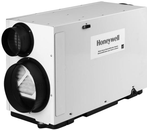
**Duct Sizing:** Use minimum 10-in. diameter round for duct lengths up to 25 ft. Minimum 12-in. required for lengths longer than 25 ft. Duct branches from the main inlet/exhaust should be minimum 10-in. round for 2-3 branches, and 12-in. round or larger for 4 branches or more.
