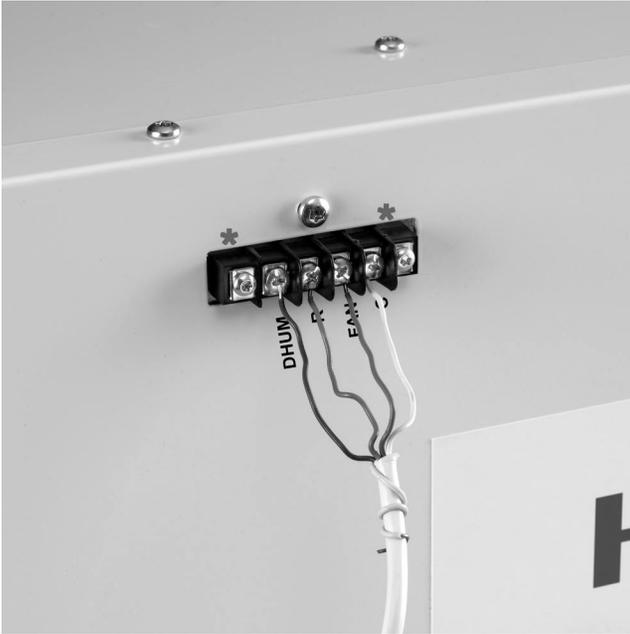
**\* NOTE:** The outer screws on the terminal block secure the block to the chassis. They are not used for wiring.
