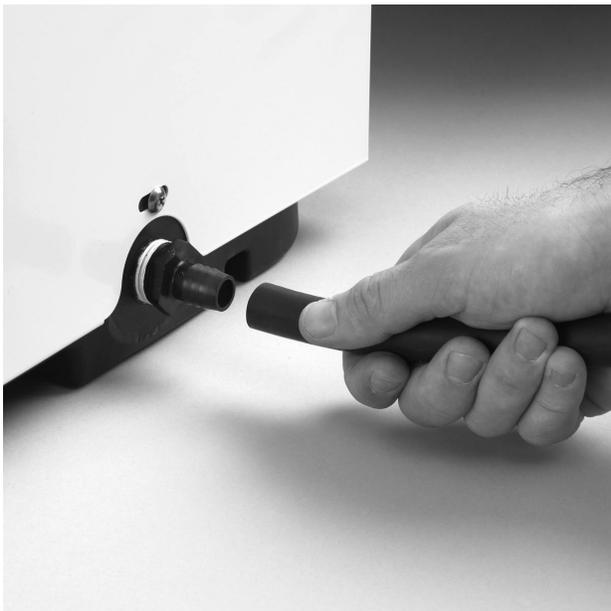
Connect 1/2-in. drain tube to male connection drain outlet. Secure drain tube to connector with hose clamp.
