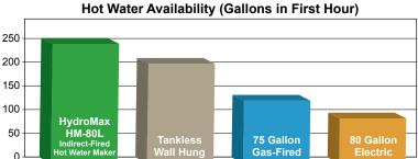
Data based on published manufacturer ratings for high-output models. Heat Input: Indirect 140,000 BTUH; Tankless 199,000 BTUH; Gas 70,000 BTUH; Electric 5500W
