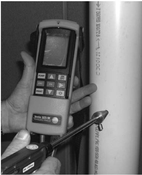
Figure 9.2: Insert Analyzer Test Probe into Test Port
