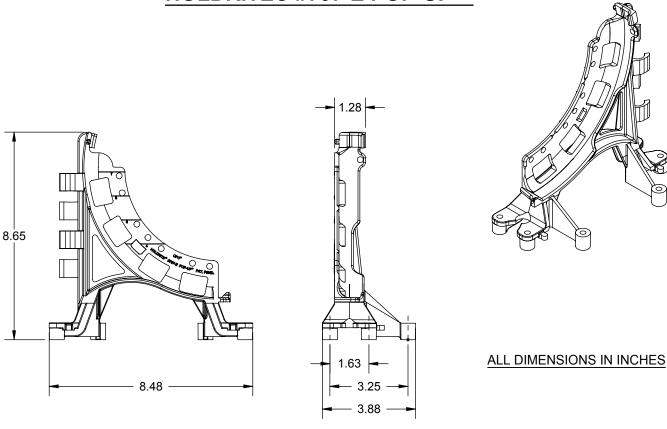
The HOLDRITE® #707-E POP-UP™ supports flexible pipe and tubing lines or rigid conduit up to 1" IPS in a 90° pattern. Ideal for positioning in-slab piping prior to concrete slab pouring. For elevated slabs, nail or screw bracket to form decking or edge form. For slab-on-grade (ground work), secure bracket with #4 rebar driven into the ground. Piping is attached to bracket with zip ties (3 included).
