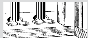
Suspension clip fasteners used at floor plate
